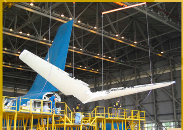
A320 Horizontal Stabilizer Replacement
